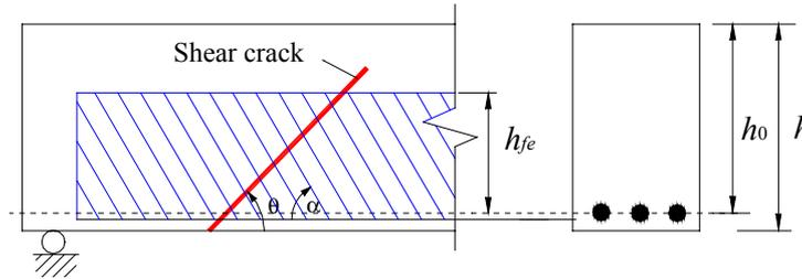
Figure 8 Effective bond height  $h_{fe}$
