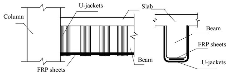
Figure 4 FRP U-jackets for flexural strengthening
