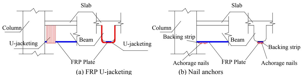
Figure 2 Additional anchors for preventing plate end debonding
