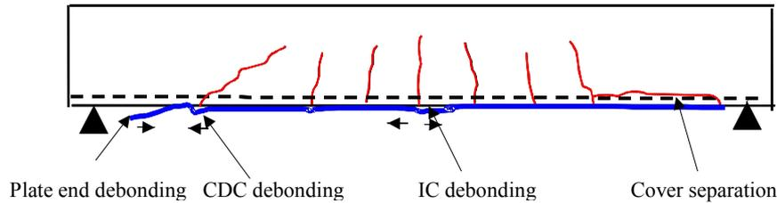
Figure 1. Debonding failure modes in flexurally-strengthened RC beams
