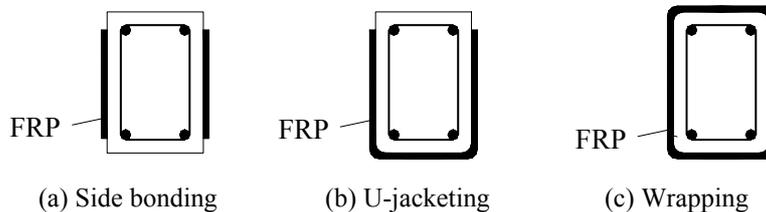
Figure 6 Common methods for the shear strengthening of RC beams
