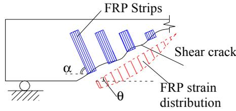
Figure 7 FRP Strain distribution along the critical shear crack
