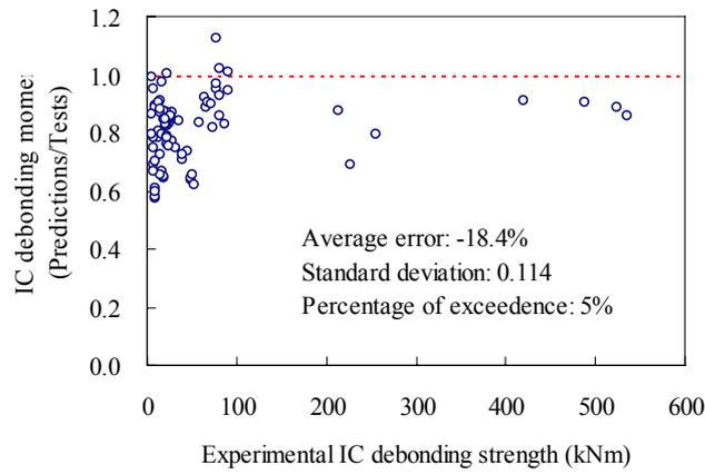
Figure 5. Adopted design model for IC debonding versus test data
