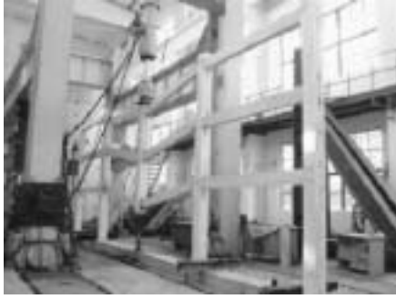
Figure 1. Collapse test of plane frame (Yi et al., 2007)
