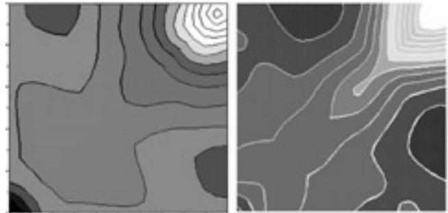
Figure 9. Concrete stress distributions of CM3
