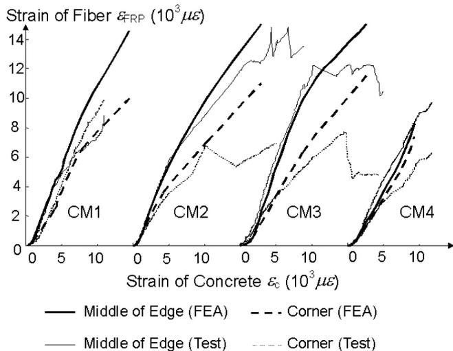
Figure 5. Strain developments of Concrete and FRP
