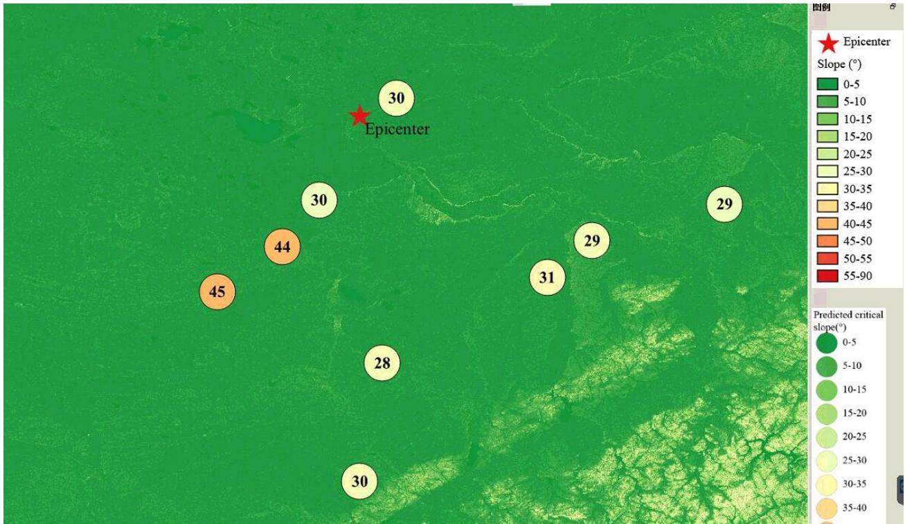
(c) The proportion of the landslide slab thickness that is saturated equals 90% Figure 4 Distribution of earthquake-induced landslide near to different stations
