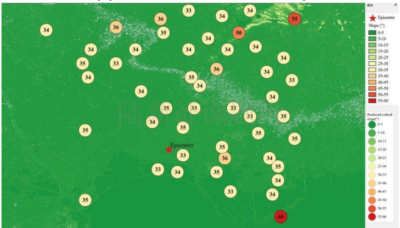
(b) The proportion of the landslide slab thickness that is saturated equals 50%
