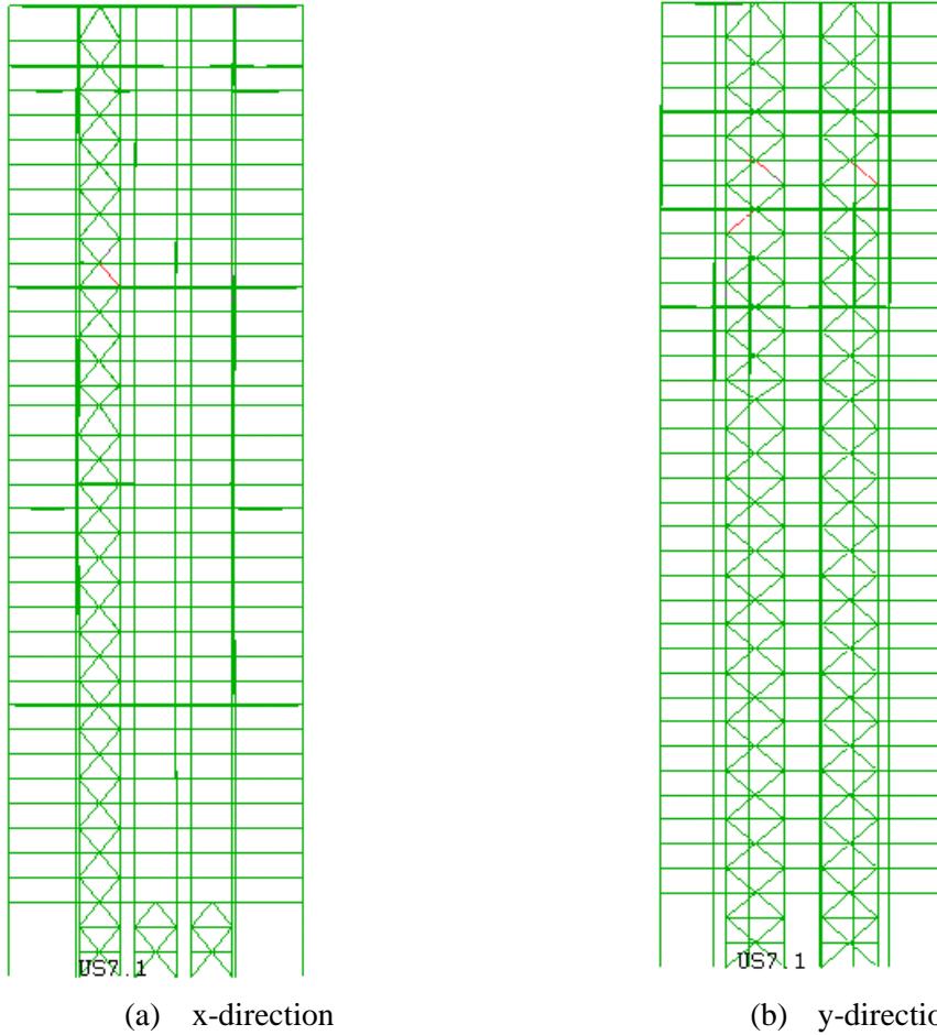
Figure 10 Damage distribution of the 37-story steel braced-frame building
